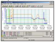
The data from the DataVU5 is read by the evaluation program and saved in an archive file. Life-cycle data management, if needed, ensures that all data throughout the lifetime of a system can be saved in an archive file. Changes to the configuration are shown separately, along with the corresponding measurement data.
