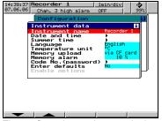
The configuration on the recorder is protected from unauthorized access by a passcode.
