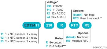
\* 9-30VDC, 7-24VAC version is also available as an extra cost option \*\* only available with 8A relay devices \*\*\* not on EDT2423
