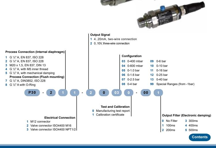
Industrial pressure transmitters for safe measurement and monitoring of many applications including gases, vapours and liquids. Designed to withstand harsh environments in the process industry.
