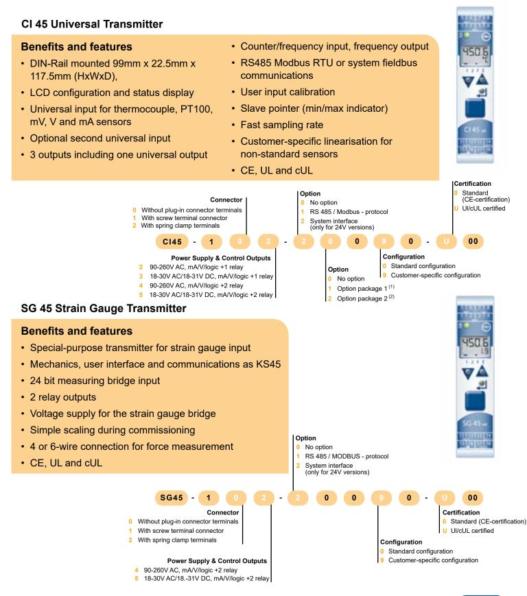
(1) Option package 1: additional universal input INP2, plus: O2-measuring; counter input; functions tare, sample & hold and integrator (2) Option package 2: additional to option package 1: digital input as optocoupler and frequency input / output
