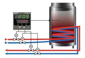
The Oenoreg+ has separate outputs to independently control the Hot and Cold water circuits.
