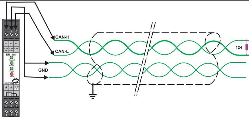
The construction of suitable cabling must be provided by the user, whereby the general cable specifications must be taken into account.
