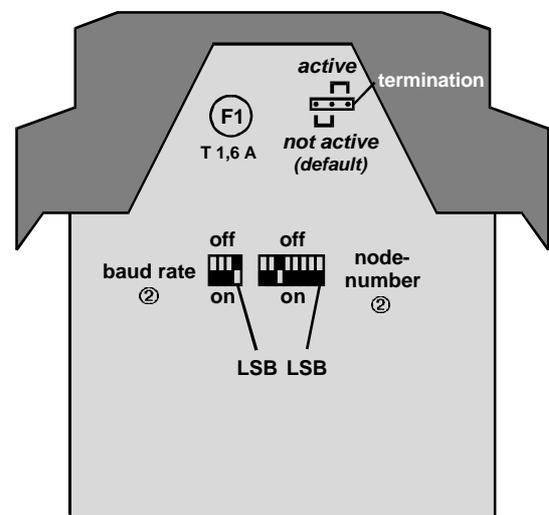
① The positions of the switches are shown in binary-code. The number at the right position corresponds to the LSB (DIP-switch-position 1), the number at the left position corresponds to the MSB (DIP-switch-position 4 or 8). To use the default-mapping of the modular fieldbus-system in full effect a node number ≤ 42 should be chosen.
