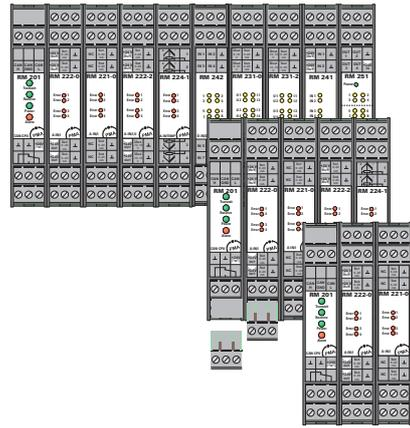
The connecting terminals can be withdrawn easily from the the modules.
