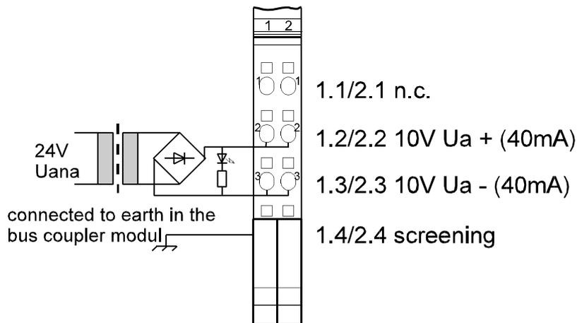
The screening earth connection must be made via the **function earth (FE)**. The screening is connected to earth only with a non-interrupted connection up to the bus coupler module provided. (The function earth is looped through all modules and connected to earth centrally at the bus coupler module.)
