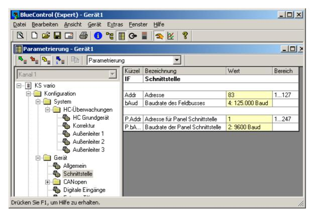
When the KSvario has been started (with valid node address), it enters the "pre-operational mode". Communication is possible via the CAN interface by means of SDOs. After configuring the bus and the device, the Master must switch the KSvario into the "operating mode" (NMT start), so that PDOs can also be used.
