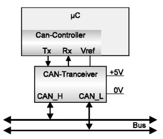
The nominal CANbus signal levels are called "Recessive" (nominal voltage of 2,5 V for CAN-H and CAN-L) and "Dominant" (nominal 3,5 V for CAN-H, and 1,5 V for CAN-L).
