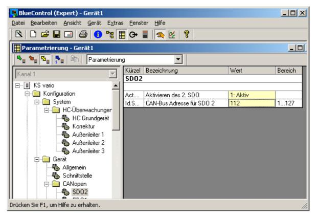
The 2<sup>nd</sup> SDO channel can be adjusted by means of BlueControl®. In the example shown, the 2<sup>nd</sup> SDO channel is activated, and the CANbus address 112 is used, so that the COB-IDs 1520 (0x5f0) and 1648 (0x670) are used. The addresses of both SDO channels must be different. The COB-ID of the 1<sup>st</sup> SDO channel is defined by the selected node address (predefined connection set).
