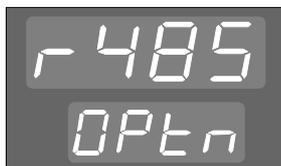
Standard RS485 Communications; maximum address range 1 - 128 (MODBUS) or 1 - 99 (ASCII).
