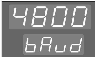
The Baud rate may be selected and confirmed as described earlier in this Section. The Baud rates available are 1200, 2400, 4800 and 9600
