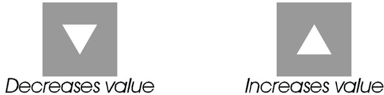
If either of these keys is held down for 10 seconds or more, the adjustment rate changes to “high speed” mode.
