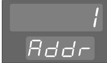
The address can be selected and confirmed in the manner previously described. Any value in the following ranges can be used, subject to the total receiver loading restrictions detailed in NOTE 2 in Subsection 1.3.12:
