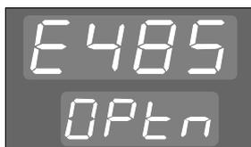
Enhanced RS485 Communications; maximum address range 1 - 255 (MODBUS) or 1 - 99 (ASCII).
