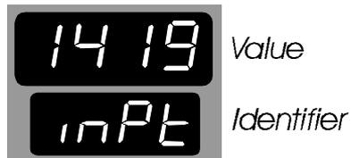
*Controller is in Configuration Mode and displays current input code*
