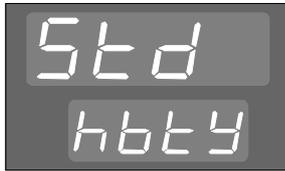
Standard Heater Break Alarm using an external current transformer (Terminals 7 and 8). This permits the use of the Low Heater Break Alarm, High Heater Break Alarm and Short Circuit Heater Break Alarm.
