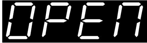
The reaction of the outputs and alarms to a detected sensor break is dependent upon the input type.
