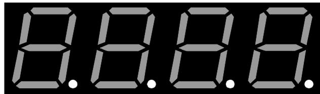
(i.e. all decimal point positions ON), parameters are at their default values, possibly due to a change in Controller configuration. To cancel this indication, adjust any Set Up Mode parameter (see below). It is recommended that all configuration parameters are finalised before any adjustments are made to Set Up Mode parameters.
