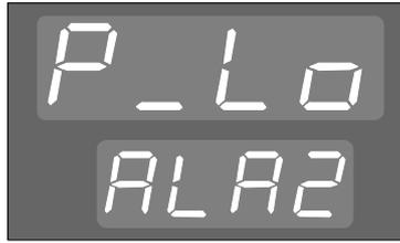
the upper display indicating the current Alarm 2 type. The alarm types available are as for Alarm 1 (see Subsection 3.3.3). The setting can be changed and confirmed as previously described. The default setting is Process Low alarm. The operation of the alarm types is shown in Volume 1, Figure 3-2.
