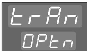
Heater Current Quick Transfer Option fitted. Terminals 11 and 12 used to instigate transfer of the current Heater Current value to the Heater Nominal Current parameter (see Subsection 1.3.6).
