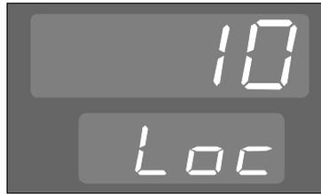
where the upper display shows the current Set Up Mode Lock Code (a Read Only display - it cannot be edited in Configuration Mode). This serves as a reminder in case the Lock Code has been forgotten (see also Volume 1, Subsection 3.2.41).
