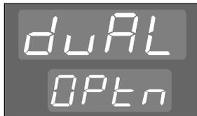
Dual Setpoint Option fitted. Terminals 11 and 12 used to select Setpoint 1 or Setpoint 2 (see Subsection 1.3.5).
