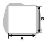
For *n* multiple instruments mounted side-by-side, cut-out A is 48*n*-4mm (1/16 & 1/8 Din) or 96*n*-4mm (1/4 Din)
