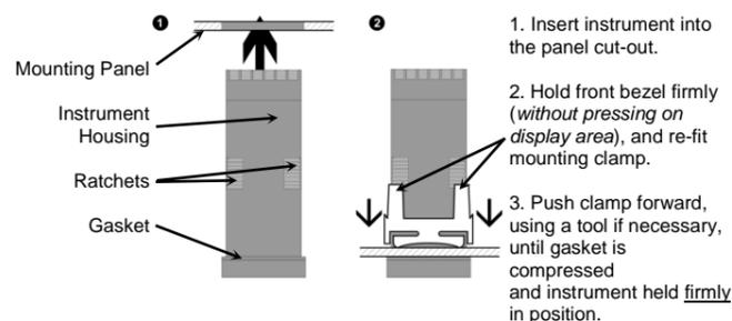
**CAUTION:** For an effective IP66 & NEMA 4X seal against dust and moisture, ensure gasket is well compressed against the panel, with the 4 tongues located in the same ratchet slot.
