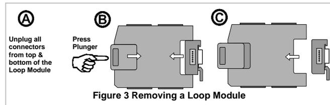
Figure 3 Removing a Loop Module
