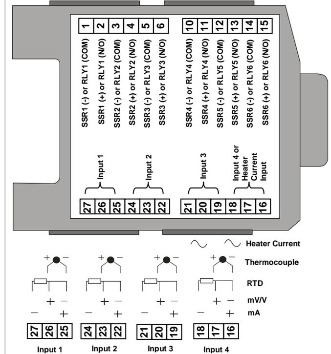
Note: Heater current input is only applicable to module variants Z3611, Z3621 and Z3651
