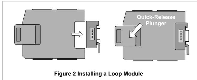
Figure 2 Installing a Loop Module
