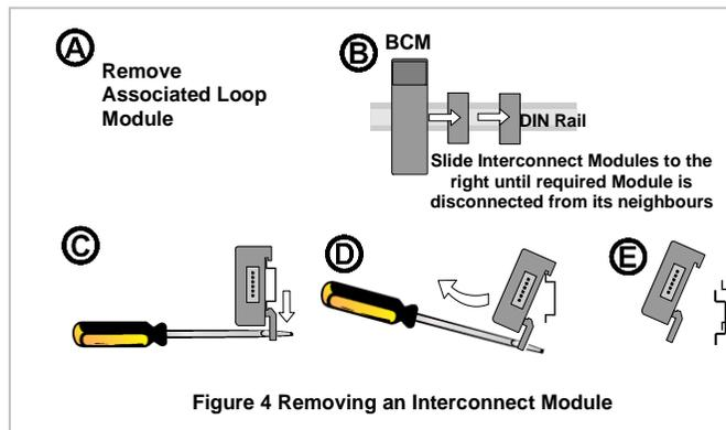
Figure 4 Removing an Interconnect Module
