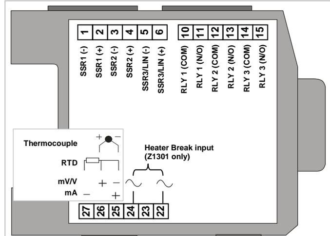
Figure 5 - Single Loop Electrical Connections
