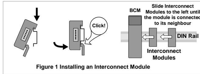
Figure 1 Installing an Interconnect Module
