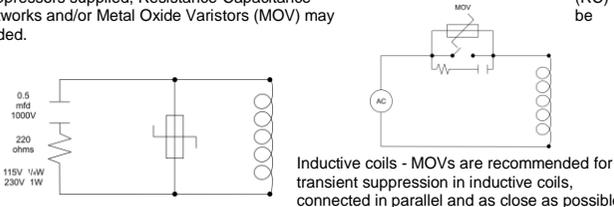
Inductive coils - MOVs are recommended for transient suppression in inductive coils, connected in parallel and as close as possible
