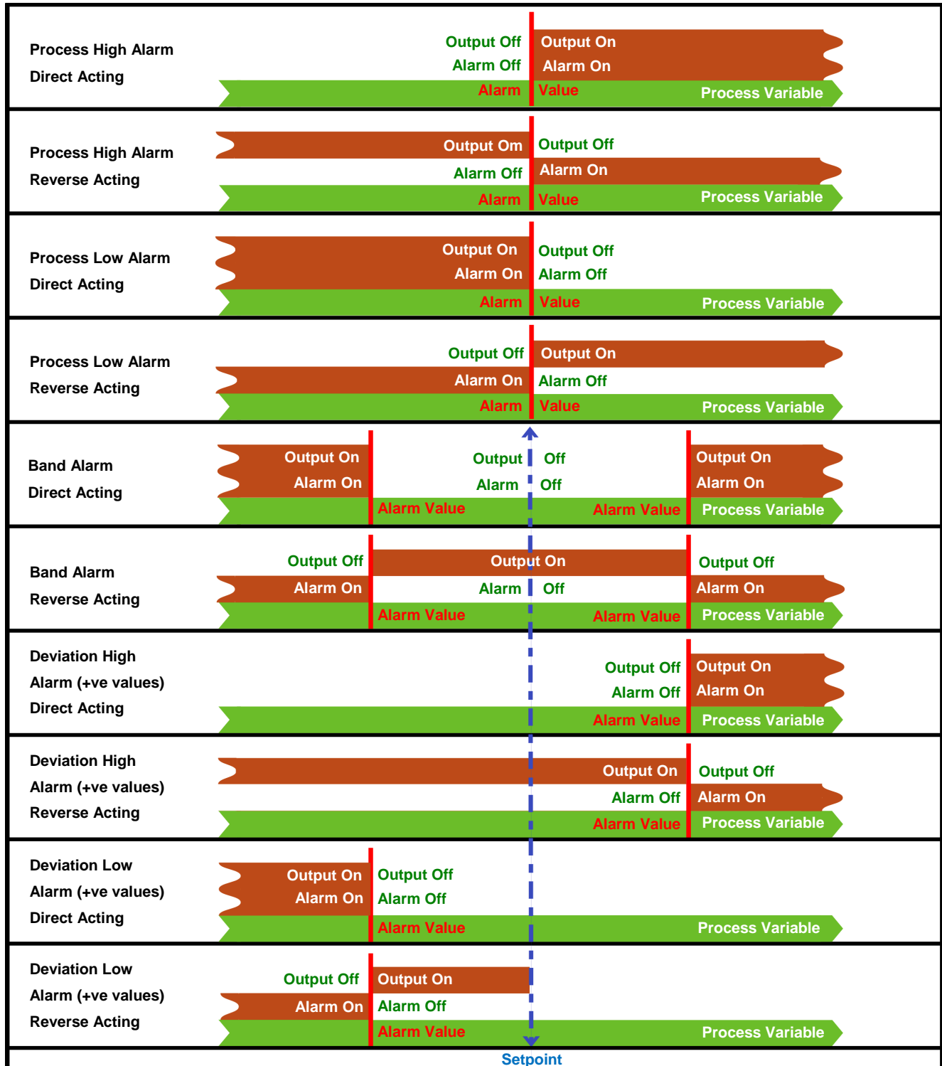
Figure 64. Alarm Operation
