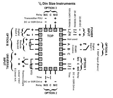
The RSP (Option A) or Remote Setpoint Input (Option B) is used for the Wine Density reading
