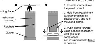
CAUTION: For an effective IP66 seal against dust and moisture, ensure gasket is well compressed against the panel, with the 4 tongues located in the same ratchet slot
