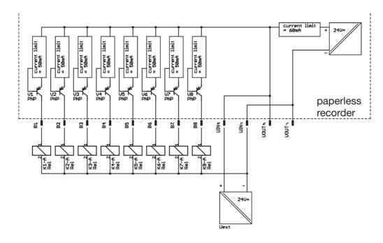
Triggering of external relays via internal supply voltage:
