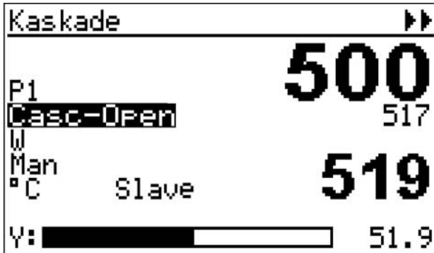
Fig. Cascade controller with open cascade
