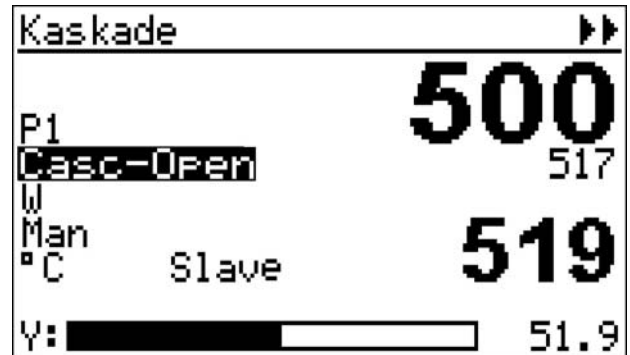
Fig. 33 Cascade controller with open cascade
