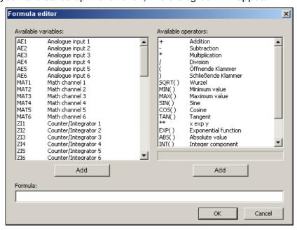
In the left window you can select the required signal, in the right window the required operator, and enter them into the formula by activating the corresponding button ( Add ). Instead of using Add , you can also make a selection by a double-click with the left mouse button.
