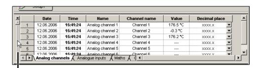
Position the mouse pointer here, and, holding the left mouse button down, shift the Teleservice window to a different position.
