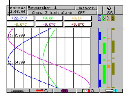
By using the parameter  $Parameterization \rightarrow Diagram \ view \rightarrow Signal \ type$  (or the button), it is possible to select whether, in addition to the analog channels, the event traces are to be displayed as well. The contents of the header are determined by means of the parameter  $Parameterization \rightarrow Diagram \ view \rightarrow Channel \ representation$  (or the button).
