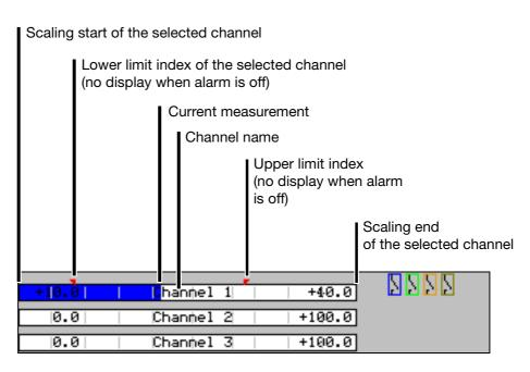
Use the parameter *Parameterization* → *Diagram view* → *Channel indication* to select which bar graph (from which channel) is to be displayed.
