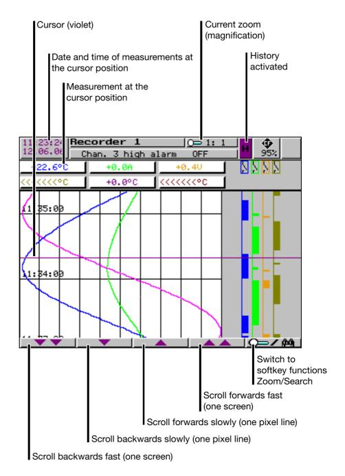
Using these softkeys, the measurement data display can be scrolled (shifted) on the screen within the measurement data stored in the internal memory.
