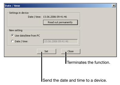
The set button is used to make date and time settings for a device. This function uses the information in the "New setting" selection as the basis for adjustment.
