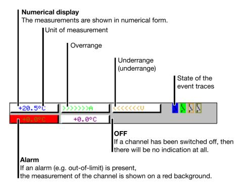
Selection and visual presentation of the channel line can be controlled through the parameter  $Parameterization \rightarrow Diagram\ view \rightarrow Channel\ represent.$  or by using the Arameterization key.
