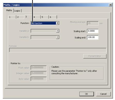
You must edit the input fields "Variable a", "Variable b" or "Time for moving average" if one of the standard functions (difference, ratio, humidity, moving average) has been set.
