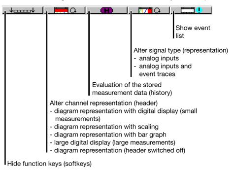
If the paperless recorder is equipped with "Counters/Integrators" (option), the symbol for indicating the counts will now appear below the softkey on the right, the symbol for showing the event list is shifted to the counter display.
