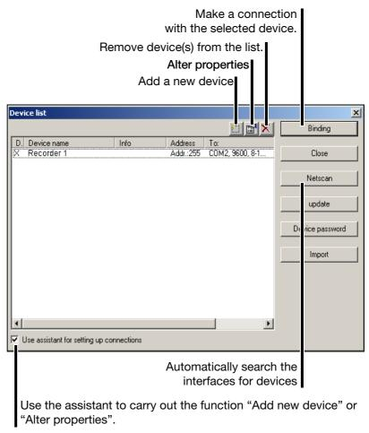
Use the Binding button to make a connection to a device. By using the Ctrl key on the PC keyboard and the left mouse button, you can select several devices at the same time (only for deleting devices from the device list).
