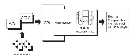
The measurements from the analog inputs are acquired continuously in a 250msec sampling cycle, and then stored in the main memory. These measurements also serve as the basis for limit monitoring.
