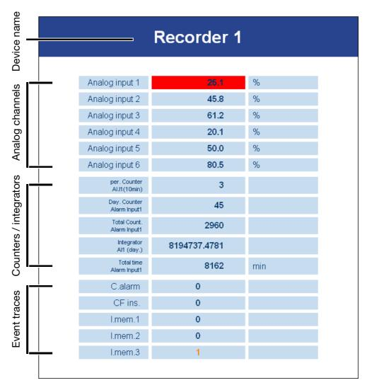
The variables that are shown are acquired and displayed automatically by the webserver. The latest data are read out of the instrument every 5 seconds. Any limit infringements show a red background. A maximum of 6 channels (analog or math channels), up to 6 counters or integrators, and a maximum of 6 event traces.
