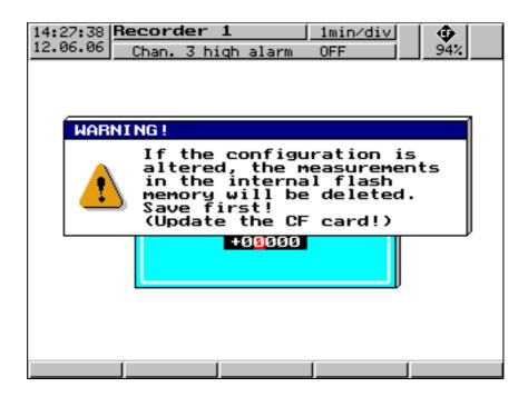
After the password has been entered in the *Configuration* menu, an additional security query will appear. You will only be able to gain access to the parameters when you have confirmed the the query with **ENTER**.
