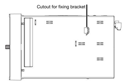
\* Push the fixing brackets up against the back of the panel and tighten them evenly.
