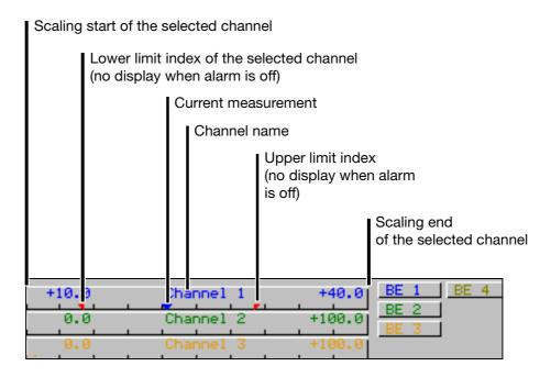
Which scaling (on which channel) is to be displayed can be selected through the parameter  $Parameterization \rightarrow Diagram view \rightarrow Channel indication.$
