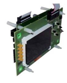
Having established the requirements of the oven, West Control customized a more cost-effective temperature control component with a controller built to fit exactly the existing oven(s), programmed to ensure that optimum temperature was restored as quickly as possible. The result of this customization is that the performance of the oven has been maximized, energy has been saved and ease-of-use improved.
